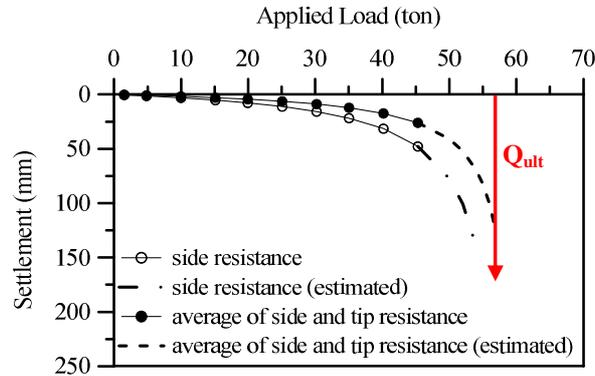
**Figure 5.** Estimation of  $Q_{ult}$  using load-settlement responses Afyon city site
