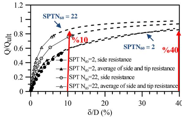
**Figure 8.** The normalized load-settlement responses for representative  $N_{60}$  values of 2 and 22 blows/30 cm
