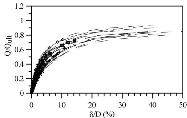
**Figure 6.** Available normalized field load tests data
