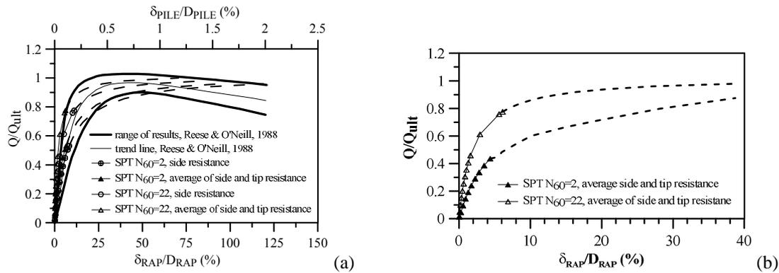
**Figure 9.** a) Comparison of normalized load-settlement curves for RAP elements and Reese & O'Neill (1988) Method, b) normalized load-settlement for SPT  $N_{60}=2$  and 22 blows/30 cm
