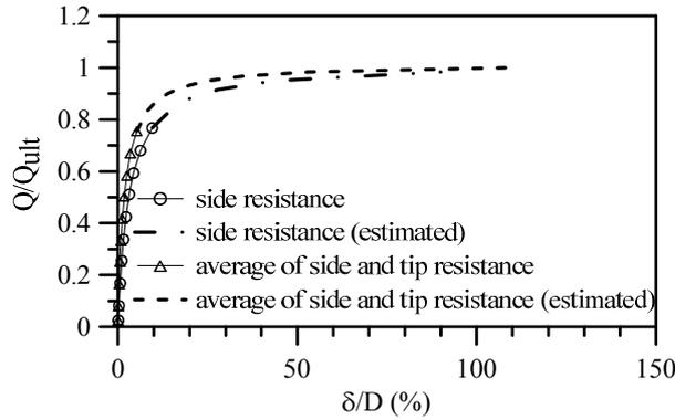
**Figure 7.** The graphs of normalized load-settlement (SPT  $N_{60}$  =9 blows/30 cm)
