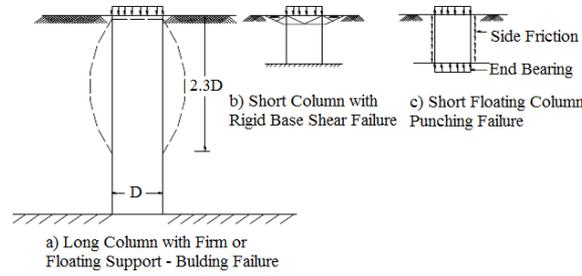
**Figure 1.** Failure mechanisms of a single stone column in a homogeneous soft layer (Barksdale and Bachus, 1983)
