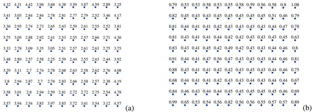
Figure 12. a) Vertical load ratio for RAPs under a 60 cm thick raft and flexible foundation b) Vertical stress ratio for soils beneath foundations in between RAPs for a 60 cm thick raft and flexible foundation
