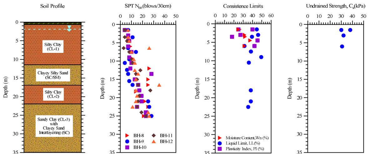
Figure 2. Generalized soil profile and a summary of laboratory test results
