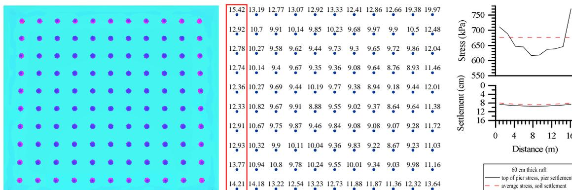
Figure 8. Vertical load distribution (in tons) on RAPs under 60 cm thick raft
