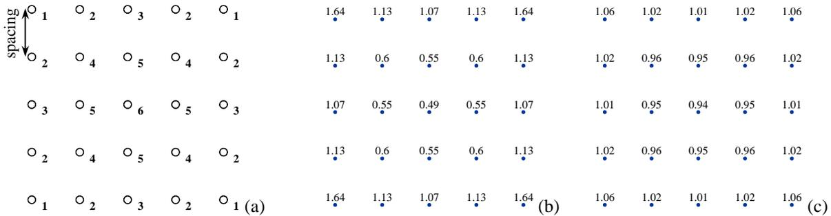
Figure 10. a) Identification of piles in 5x5 square groups, vertical load distribution 5x5 pile group for b) rigid cap c) equally loaded, Poulos and Davis (1980)
