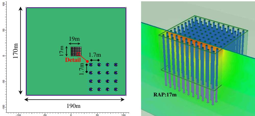
Figure 7. 3-D finite element mesh of the RAP-improved raft foundation
