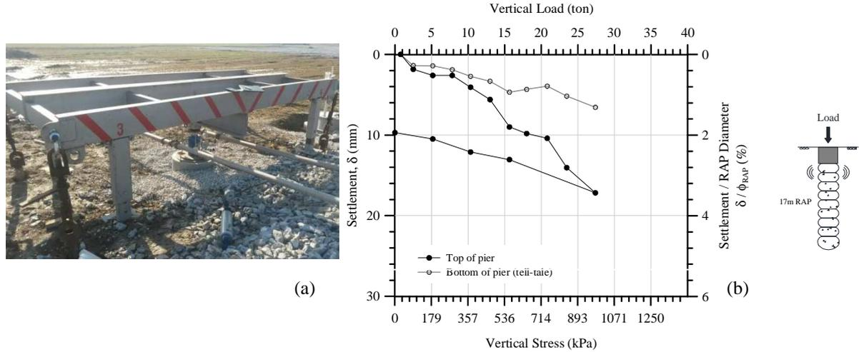
Figure 4. a) The single RAP load test set-up b) the field load test results
