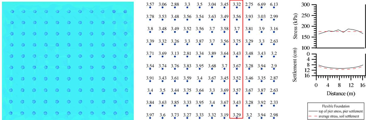
Figure 9. Vertical load distribution (in tons) on RAPs under a flexible foundation
