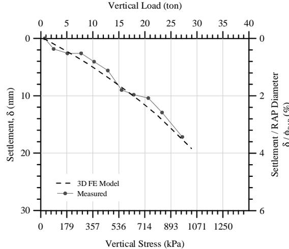
Figure 6. Comparison of measured and calculated pressure-settlement curves
